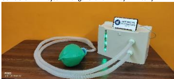
Low-cost & Portable Emergency Use Ventilator
